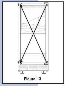
All Electrolux units may be left or right hand opening. The door opening is easily reversed by moving the hinge hard-ware to the opposite side (see **Figure 13**).
